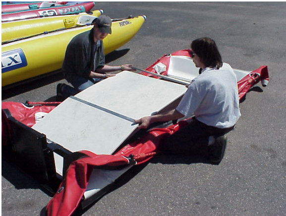
STEP 3, 4 and 5: Insert middle section, join with floor joiners and press down. Place the edge of the floorboard down under the floor rubber as shown along both sides of boat.
