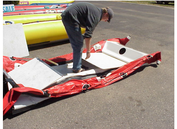
STEP 3, 4 and 5: Insert middle section, join with floor joiners and press down. Place the edge of the floorboard down under the floor rubber as shown along both sides of boat.
