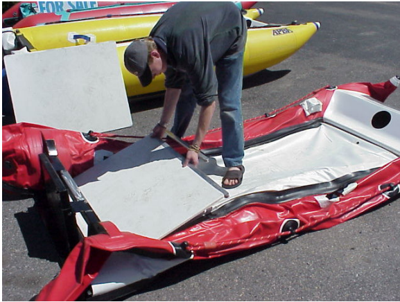
STEP 3, 4 and 5: Insert middle section, join with floor joiners and press down. Place the edge of the floorboard down under the floor rubber as shown along both sides of boat.
