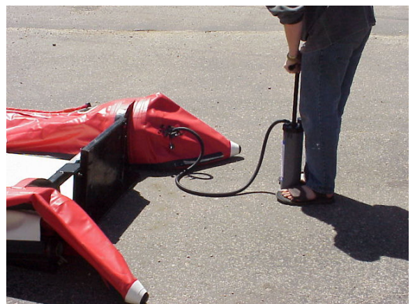
Step 6: Inflate using pump included to 6 PSI
